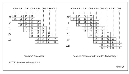
Figure 16-1. Embedded Pentium® Processor Pipeline Execution
